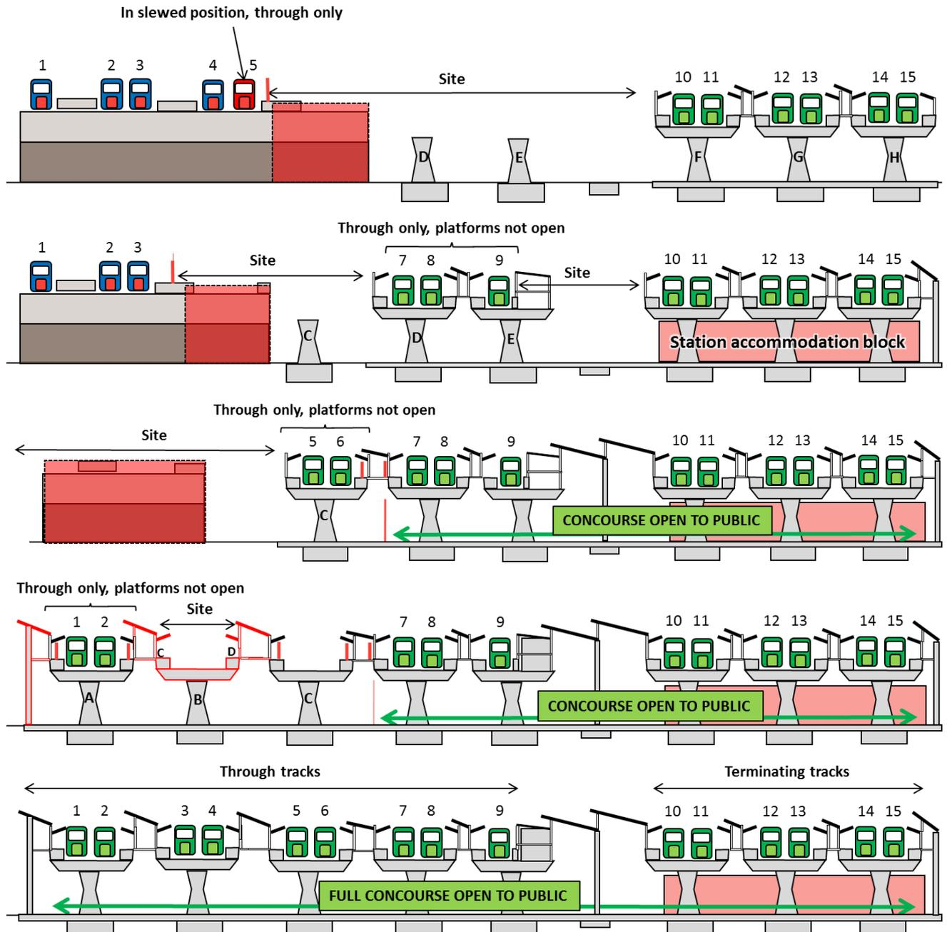
Figure 3 – construction sequence (Costain)
