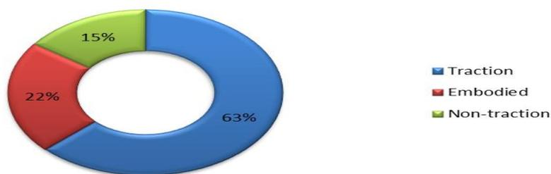
Figure 1 – whole system carbon footprint of rail industry
