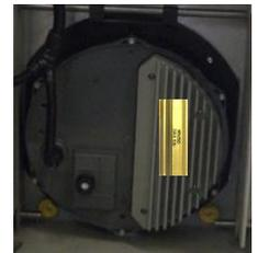
Fig.4 LED module with pluggable resistor. Recommended position.
