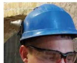
The future for noise monitoring at LBSR was further enhanced by the addition of personal noise dosimeters. These conical gadgets are designed to be attached to a hard hat and record noise throughout a shift allowing data analysis of personal noise levels of operatives in different trades on site.
