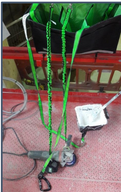
Tool tethering basket with individual tool tethers
