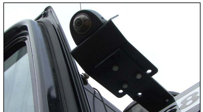
The 360° degree camera system above that interlinks pictures from multiple cameras that can pick up a pedestrian from a maximum distance 5m to a minimum of zero in all directions
